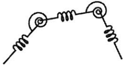
Figure 69. The inner mechanics of a finite-element model for physically simulating a hair-like filament: linear springs alternate with torsional ones.
