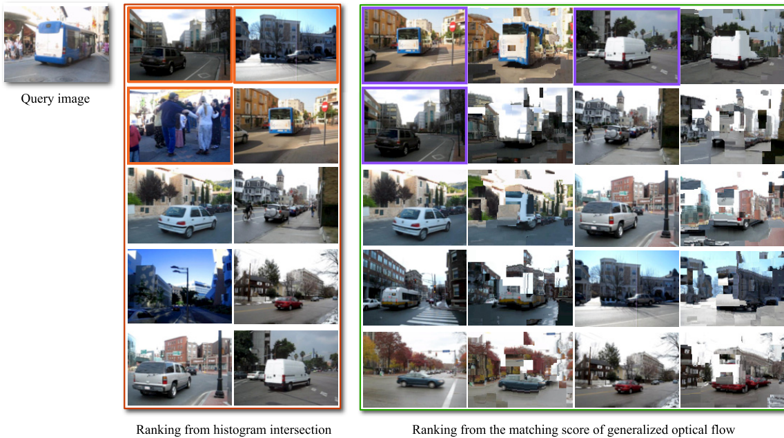
Fig. 15. SIFT flow typically improves ranking of the nearest neighbors. Images enclosed by the red rectangle (middle) are the top 10 nearest neighbors found by histogram intersection, displayed in scan-line order (left to right, top to bottom). The top three nearest neighbors are enclosed by orange. Images enclosed by the green rectangle are the top 10 nearest neighbors ranked by the minimum energy obtained by SIFT flow, and the top three nearest neighbors are enclosed by purple. The warped nearest neighbor image is displayed to the right of the original image. Note how the retrieved images are re-ranked according to the size of the depicted vehicle by matching the size of the bus in the query.
