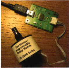
Figure 34. TouchSense PR-1000 knob with programmable detents, friction, and end points.
