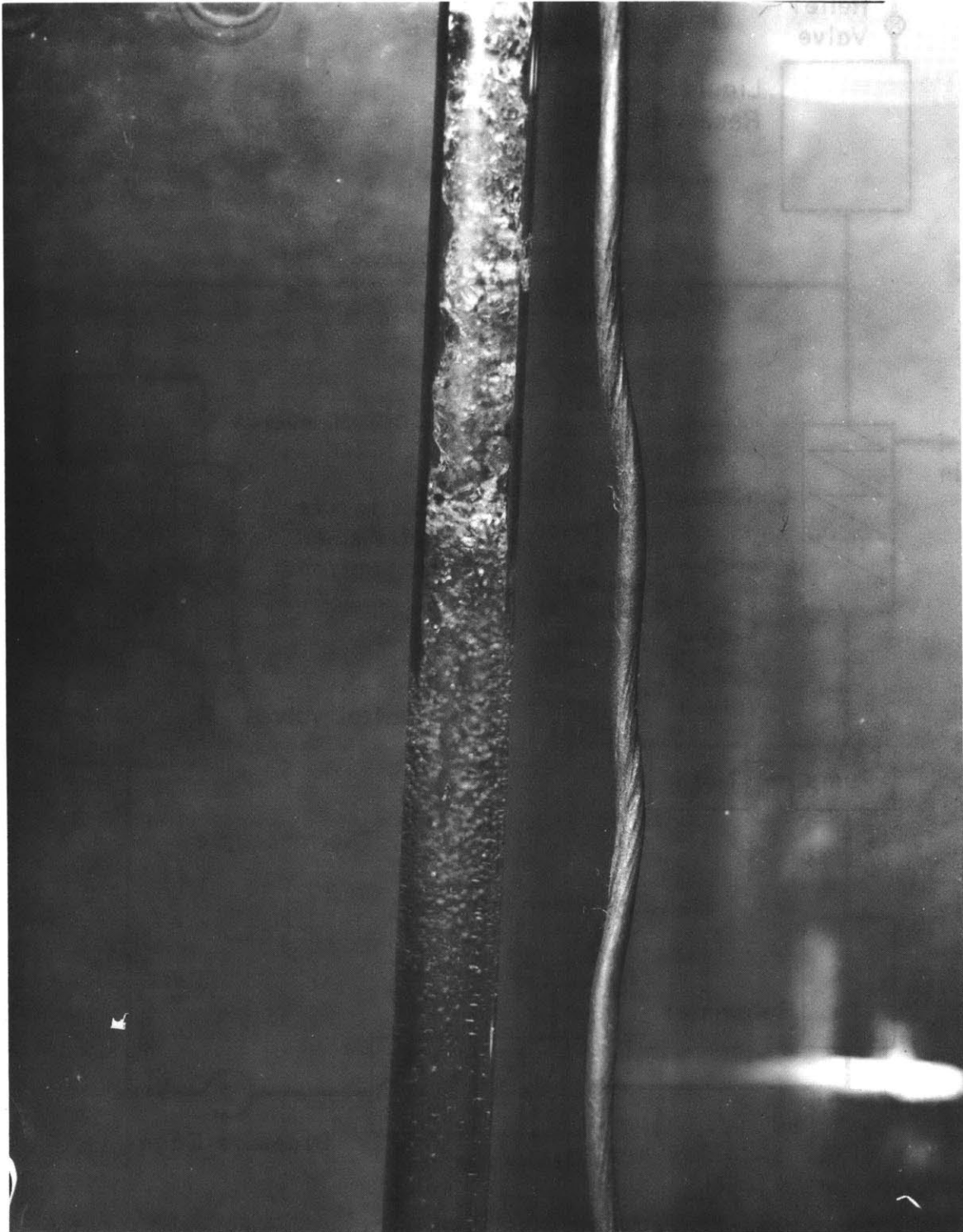
Figure 1. Photograph of Film Boiling Inside a Vertical Tube with G=6.60 \times 10^5 lbm/hr-ft 2
