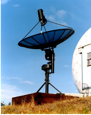
Figure 1. A view of the Small Radio Telescope, an inexpensive educational aid developed at Haystack Observatory to introduce students and amateurs to radio astronomy.
