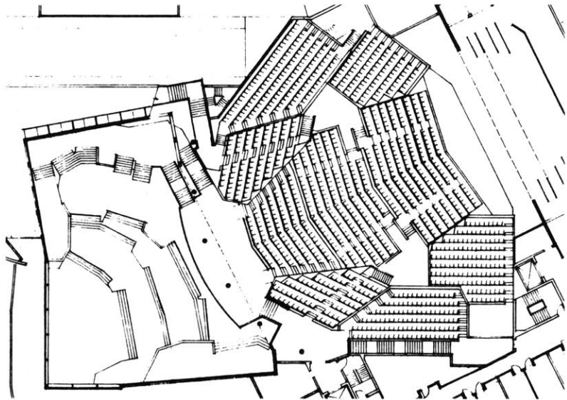
Figure 2.15 The form of the lobby steps begin to suggest seating tiers like the auditorium; this introduces the visitor to the auditorium before arriving in it, and creates a performance space of itself. The lobby experience becomes a part of the performance, or a separate theatrical venue.
