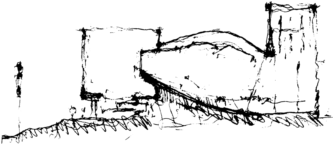
Figure 5.11 Sketch section, showing dominance of the lobby space in the spatial sequence. The steps establish continuity.
