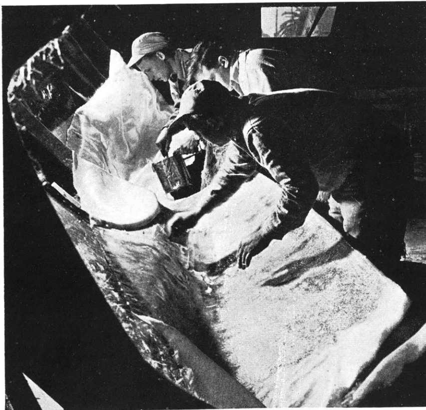
Large parts, like auto bodies and boats, are built up by hand laying cloth and mat and impregnating with resin. (United States Rubber Co.)
