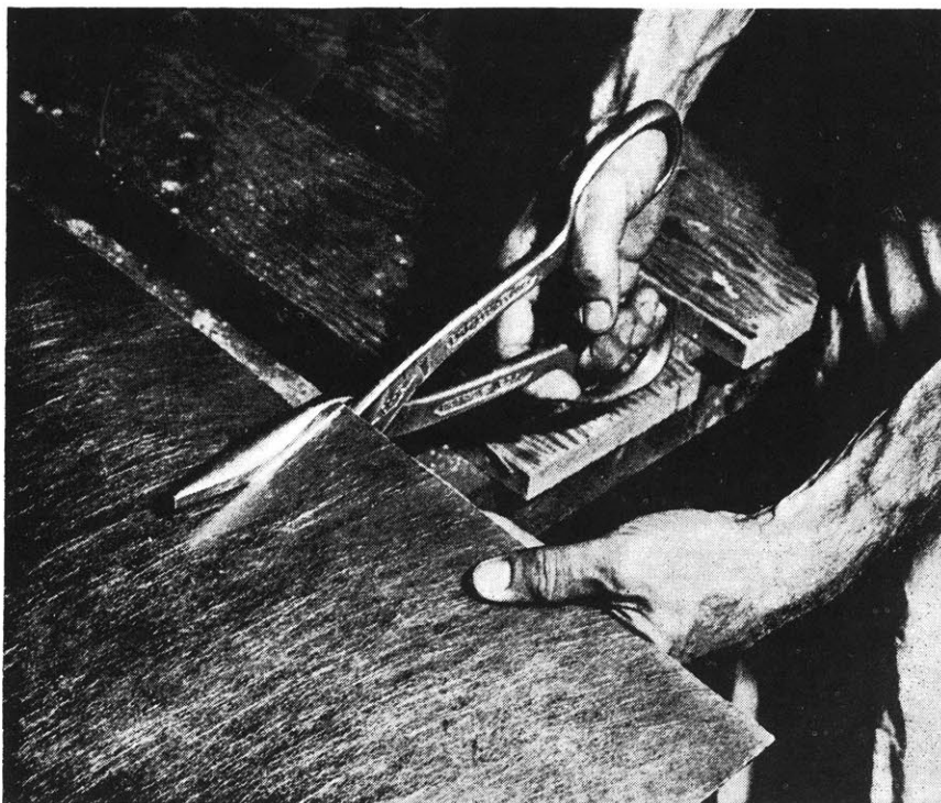
Panels cut easily with shears or standard saws. The material can also be drilled with regular tools and fastened by bolts or adhesive. (Alysinte Co. of America.)
