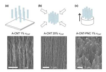
**Figure 3.** Schematic and SEMs of nanocomposite fabrication.<sup>27, 30</sup> (a) As grown CNT films with 1 *vol.*% CNTs. (b) Biaxial mechanical compression of CNTs up to 20 *vol.*% CNTs. (c) A-CNT-PNC fracture surface after capillary-driven epoxy infiltration of the CNT arrays.
