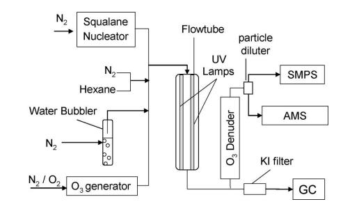
Figure 2. Schematic of the flow reactor used in the present experiments. Squalane
