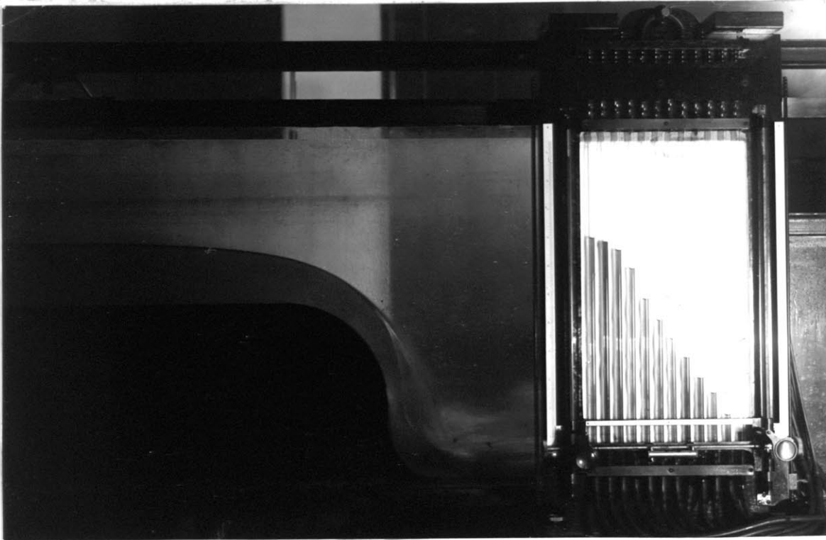
Photo 5. Discharge of 125 l/s/m, radius of curvature of downstream face 20 cm. Standpipes show pressures on weir face through entire transition.
