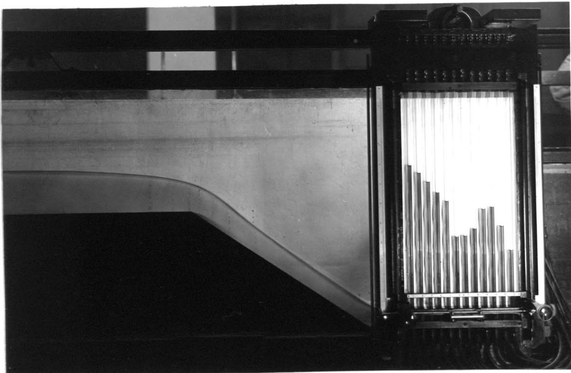
Photo 6. Discharge of 125 l/s/m, slope of weir face 1:1½; standpipes show pressures on weir floor and slope through entire transition; color shows limits of roller.
