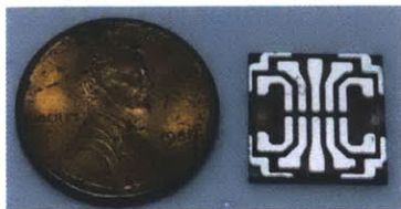
Figure 4.2. Size comparison of a coupon containing 8 solar cells on it and a 5 cent coin
