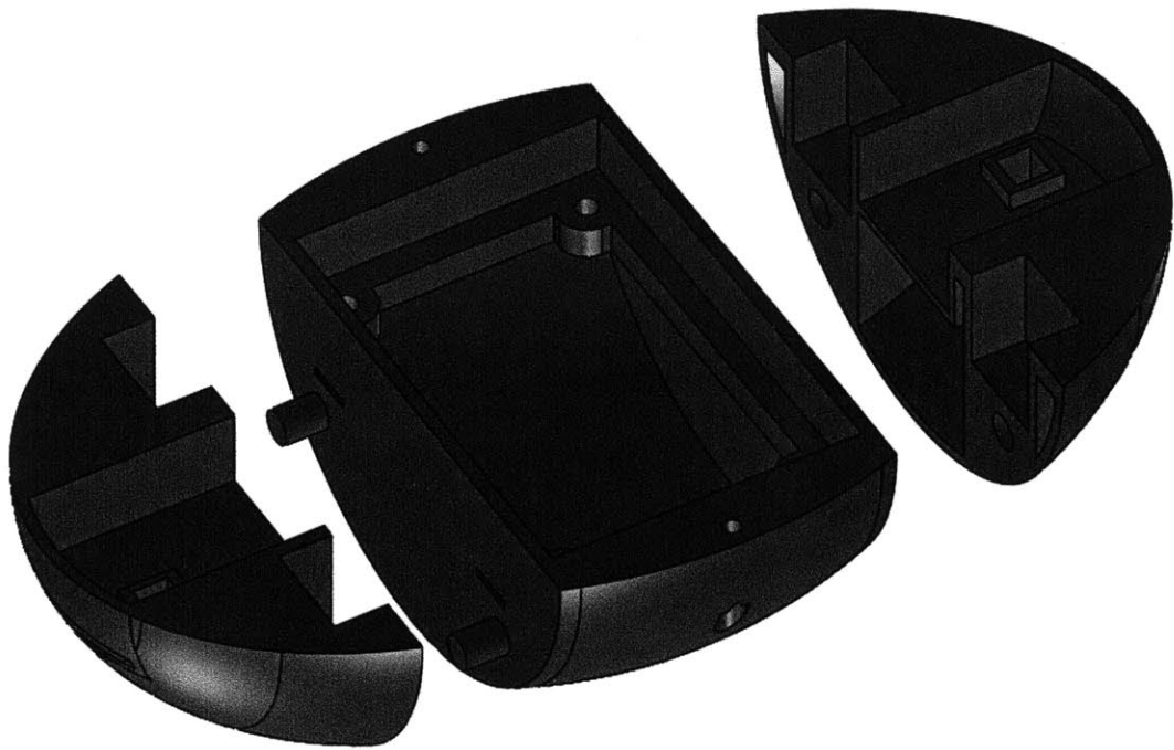
Figure 3-3: Models for the electronics-half of the robot. The central box is fabricated from waterproof material, snaps together with the two sides, and prevents free motion of the electronics.
