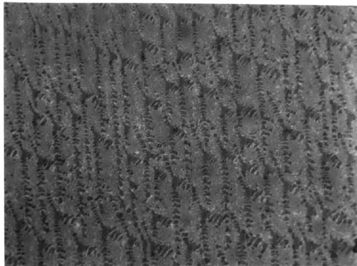
Figure 33: A vertical section through arc deposit in 38 percent copper alloy at \sqrt{q/v} = 5 . X 500 Etch \text{HNO}_3
