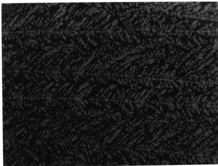
Figure 19: Horizontal section of arc deposit far from interface showing long \alpha dendrites along the length of the weld. X 500 Etch \text{HNO}_3
