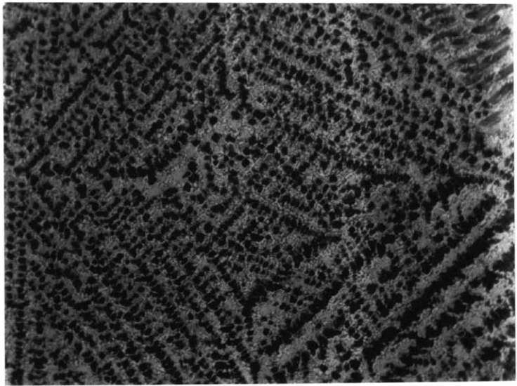
Figure 28: Horizontal section through 38 percent copper alloy chilled cast plate showing three fold symmetry in arrangement of side branches in \text{CuAl}_2 dendrites. X 50 Etch \text{HNO}_3
