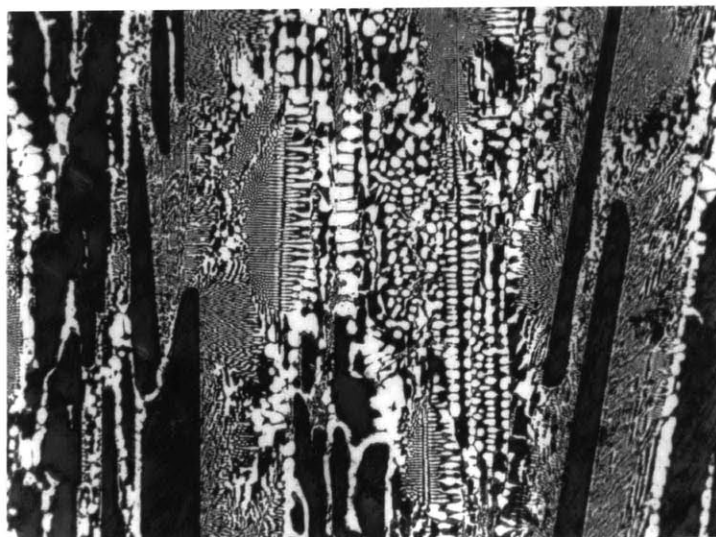
Figure 57: Vertical section through directionally slow cooled ingot of 38 percent copper alloy. Note the tendency of \text{CuAl}_2 to arrange itself in dendritic form with side branches. Behaviour like anomalous eutectic appears to be the cause. X40 Etch \text{HNO}_3
