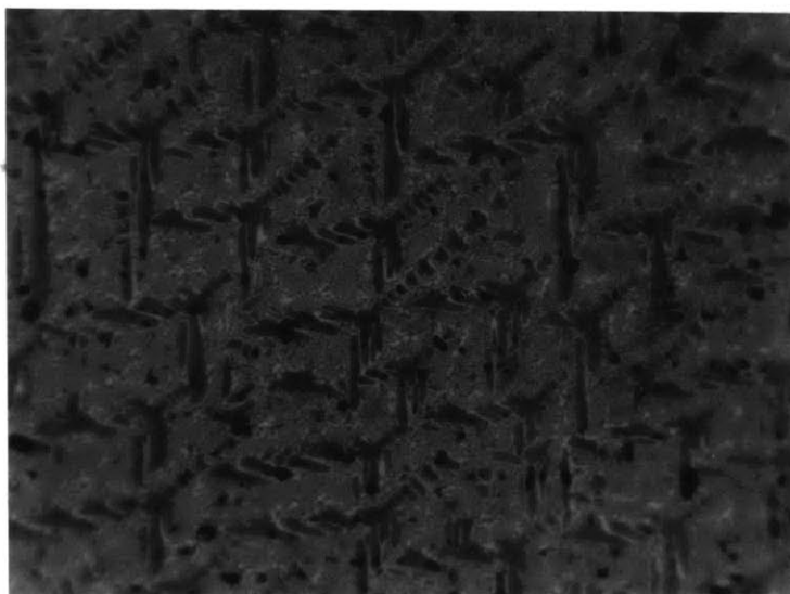
Figure 34: A vertical section through arc deposit in 38 percent copper alloy at \sqrt{q/v} = 20 . Note the large dendrite spacing compared to Figure 33. X 500 Etch \text{HNO}_3
