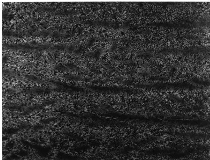
Figure 41: Vertical section through slow cooled (plaster cast) ingot of 33 percent copper alloy showing lamellar (unresolvable at this magnification) eutectic arranged in dendritic form with coarse irregular eutectic in between. X13 Etch \text{HNO}_3
