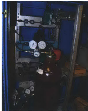
(c) Gas distribution system used to inject high purity gas into the growth chamber during reduction and growth
