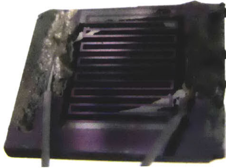
Figure 4.2: Damage to sample tested in sulfuric acid
