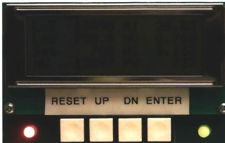
Diagnostic Display showing IRt/c mV Signal, equivalent Temperature, Setpoint Temperature, equivalent mV Signal, Reference (ambient) Temperature, Heater Voltage, Heater Current, and Amplifier Pulse Width
