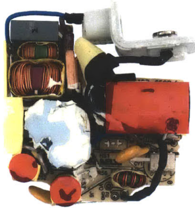
Figure 1.2: Mainboard of a 2009 Apple laptop charger with electrolytic capacitors highlighted in red
