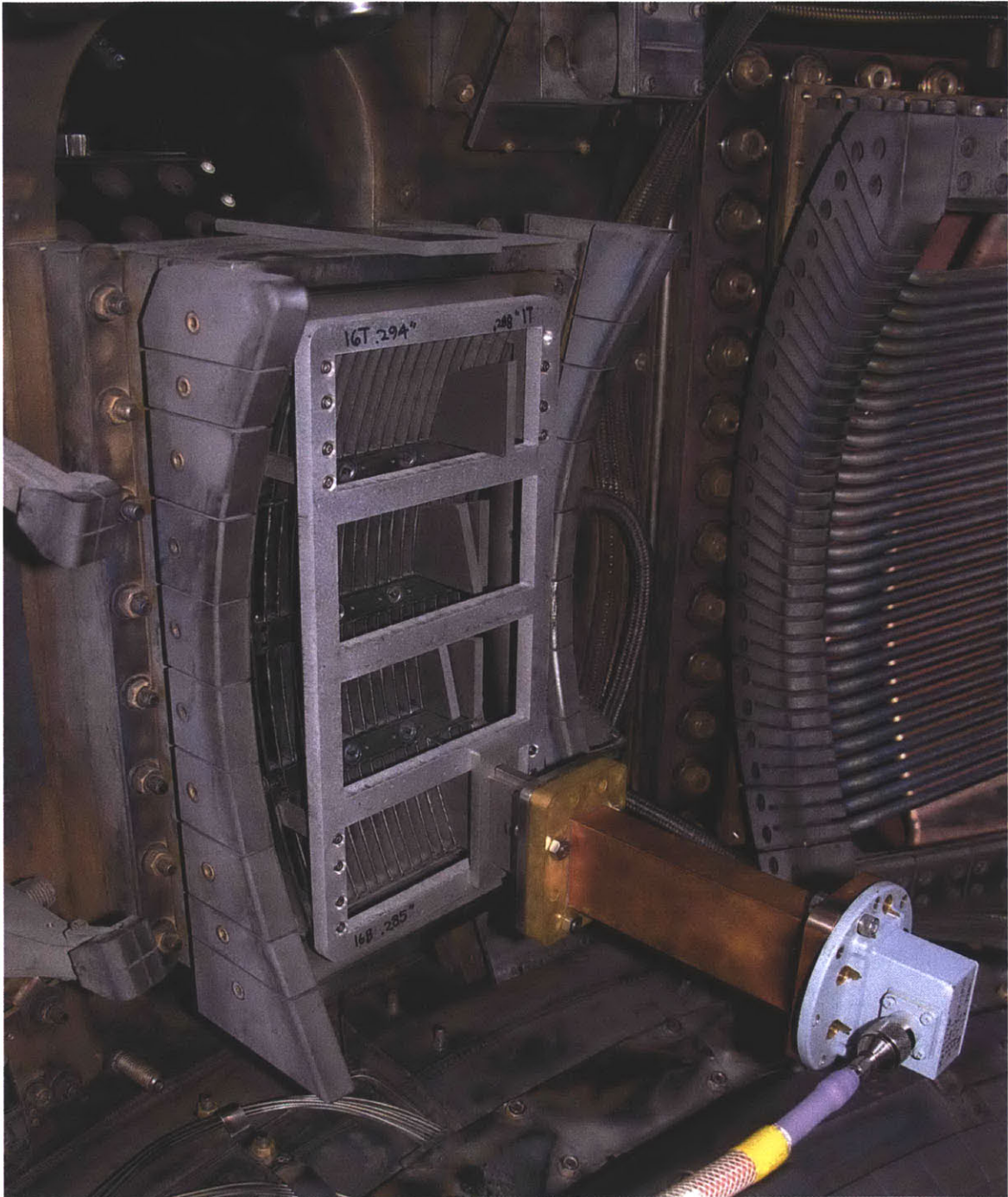
Figure 4-15: In this picture, the Oframe and the Odaptor in place, during an in-vessel calibration, at the end of the 2010/2011 campaign. While the amplitude and phase are measured by means of the Odaptor , wedge loads are inserted in the other waveguides.
