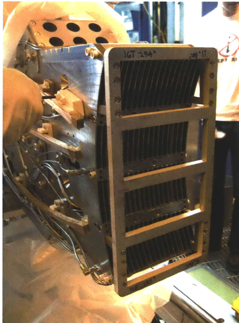
Figure 4-14: On the left, CAD drawing of the Oframe which is used to set the reference plane for the phase measurements on the launcher. Shown in black is also the Odaptor , as it would be used in combination with the fixture. On the right, the fixture once is installed on the launcher.
