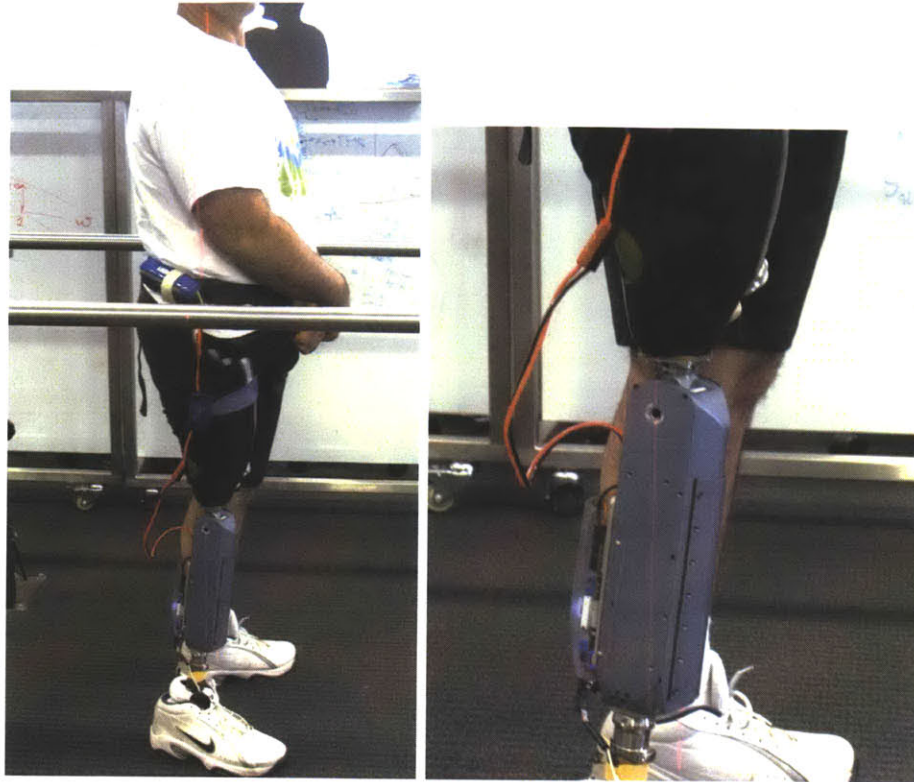
Figure 6.4-Fitting of active knee prosthesis. Adequate alignment with laser guide. Location: Biomechatronics research group at MIT Media Laboratory.
