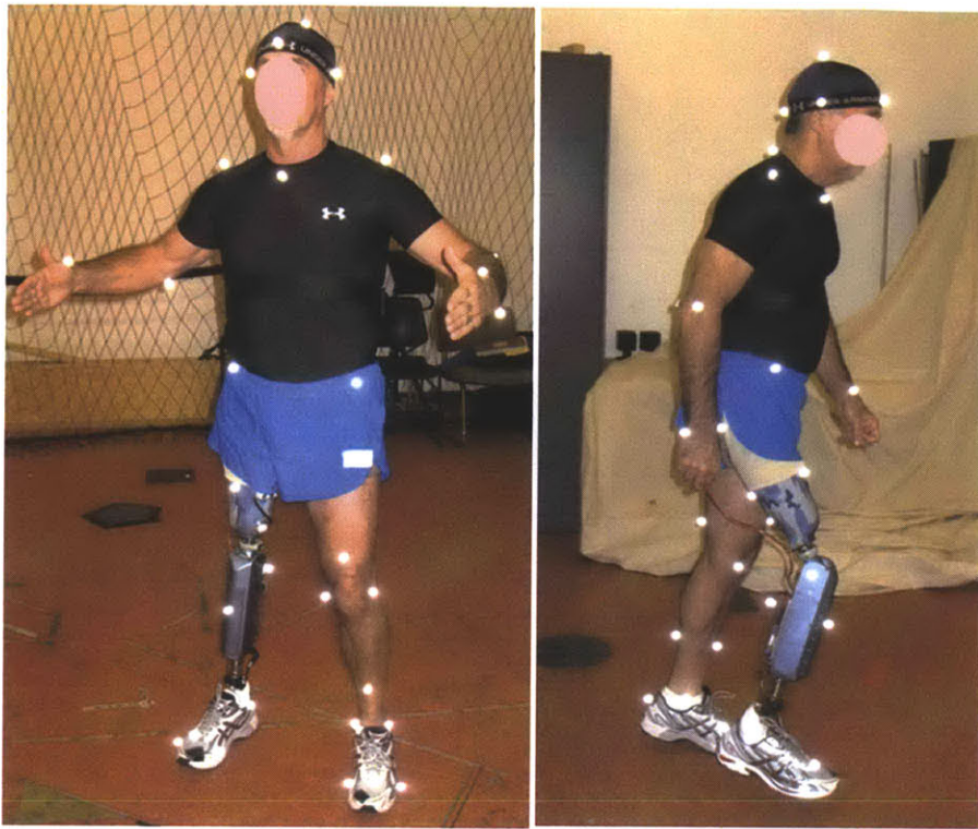
Figure 6.6-Transfemoral amputee wearing the biomimetic active knee prosthesis, instrumented with reflective markers at the motion capture laboratory .
