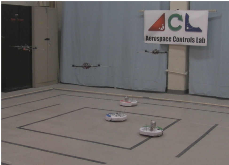
Figure 4-5: Real-time mission planning for a heterogeneous networked team using the CBBA planning framework (Aerospace Controls Lab, MIT).
