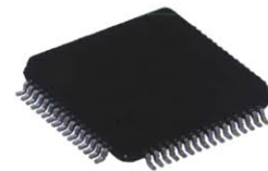
▲ ARM 32-bit microcontroller (STM32F106RET6)
