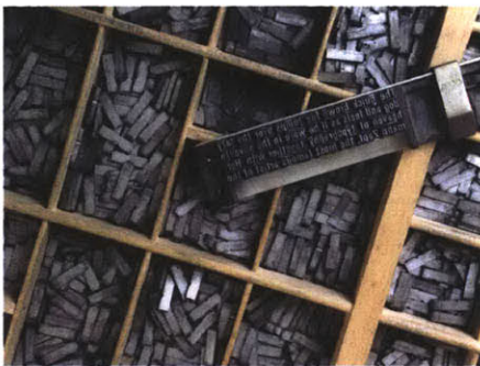
▲ Type carriage for a press printer. This type of printer is a descendent of the first Gutenberg printer and was the standard until inkjet printers became available.
