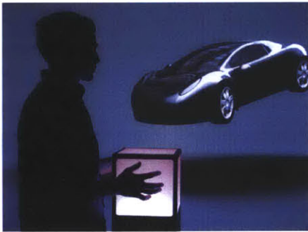
▲ Cubtile by Rivière et al. enables users to manipulate 3D models by means of a multi-touch cubic input device.
