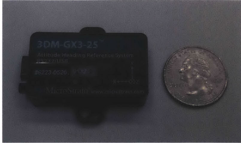
Figure 3-3: The 3DM-GX3-25 Attitude Heading Reference System.
