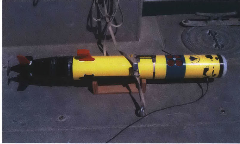
Figure 3-2: REMUS-100 vehicle strapped to the deck of the R/V Tioga prior to deployment on April 26th.
