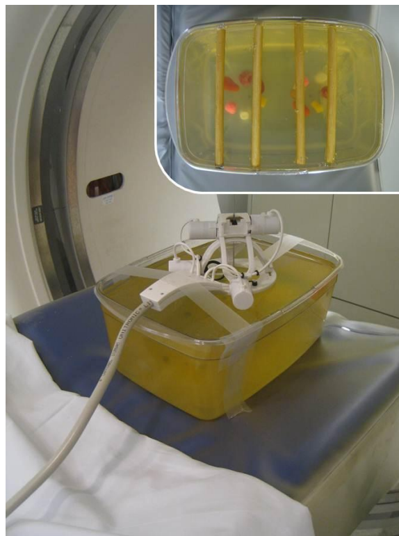
Figure 57 – Testing the gamma interface on gelatin phantom. Soft targets are under wooden dowels simulating ribs.
