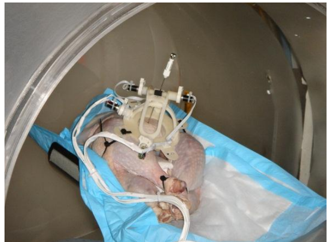
Figure 44 – Testing with turkey tissue. Plastic ties strap the robot to the turkey.
