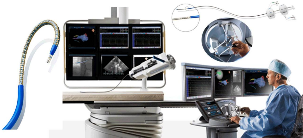
Figure 16 – Hansen medical system showing (left to right) the catheter, the patient side base unit and the operator interface with detail of the hand piece, [61].
