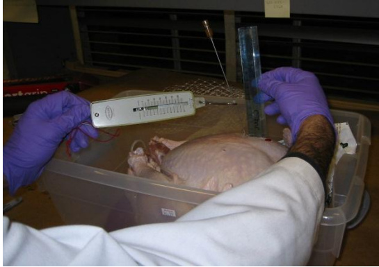
Figure 32 – Measuring force required to angulate a needle previously inserted into a turkey breast.
