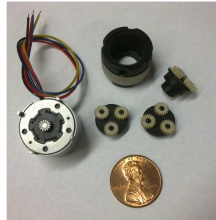
Figure 50 – Detail of Saia motor and gearbox.
