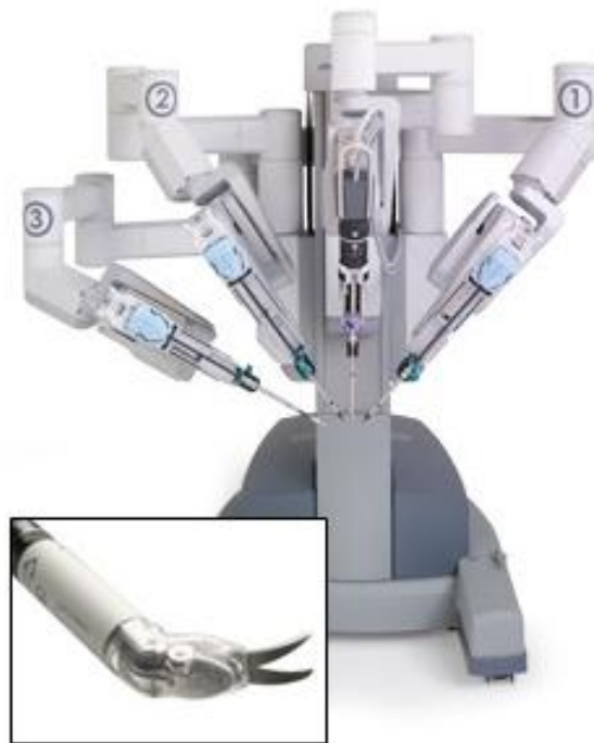
Figure 17 – da Vinci patient-side cart and sample EndoWrist attachment [65].
