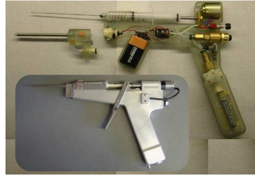
Figure 74 - Student prototype with inset showing second generation prototype.
