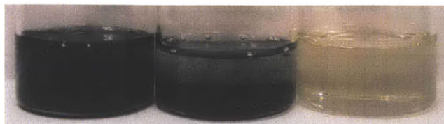
Figure 1.3. Photograph of uncured epoxy resin taken 30 minutes after mixing with 1 weight % EpCNT2 (left) and 1 weight % MWNT (center). The neat epoxy is shown (right).
