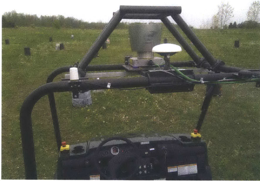
Figure 4.3. LIDAR, GPS, and communication antennae
