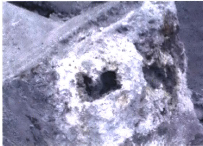
Figure 5. A photograph of aluminum dross byproduct (Urbach 2010).
