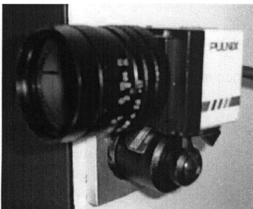
Figure 3-3: Pulnix camera, mounted
