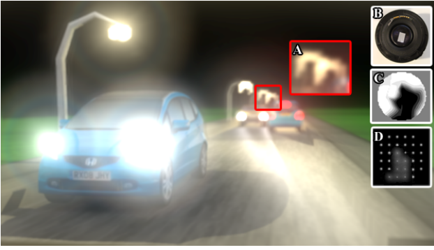
Figure 7: Rendering features using measured PSFs from a simulated cataract on a DSLR camera: (A) “Bokeh” effect, the cataract shape projected from out-of-focus bright light sources; (B) picture of the simulated cataract; (C) the estimated attenuation map; (D) the estimated PSF map; Cataract spots scatter light generating large glare patterns. Depth information captured from the z-buffer. Camera aperture of 4mm.
