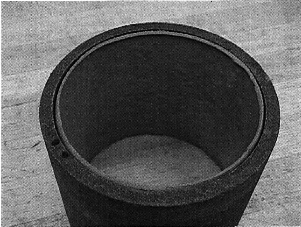
Figure 4-2: Picture of Mudcake Inside the Filter
