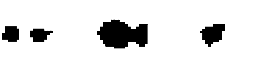
Figure 5.1: This is the set of slices used to create the volume. The shapes were chosen so as to be irregular, yet identifiable in the output. The volume was composed by using purely white images for slices 1-6 and 24-30, the first image in the set for slices 7-11, the second image in the set for slices 12-18, and finally the last image for slices 19-23.
