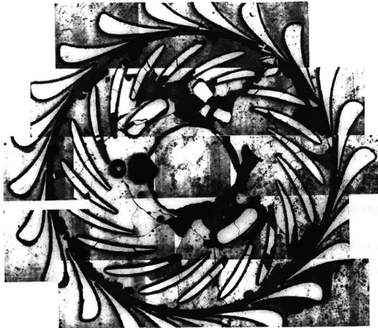
Figure 4-12: Assembly of optical pictures of the crashed rotor after crashing at 510,000 RPM (first die of MCBR1 build)
