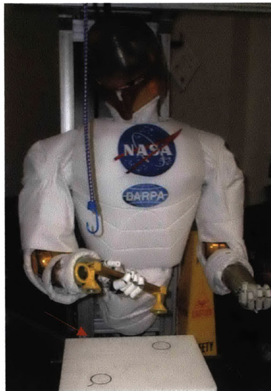
Figure 7.3 Photograph of integrated handrail task set-up
