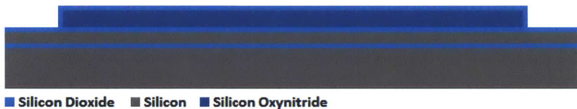
Figure 45 - Upper silicon dioxide cladding is deposited
