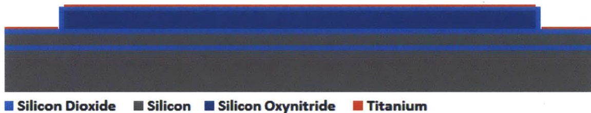
Figure 45 - Titanium removed on sidewalls corresponding to inputs and outputs of the waveguides.
