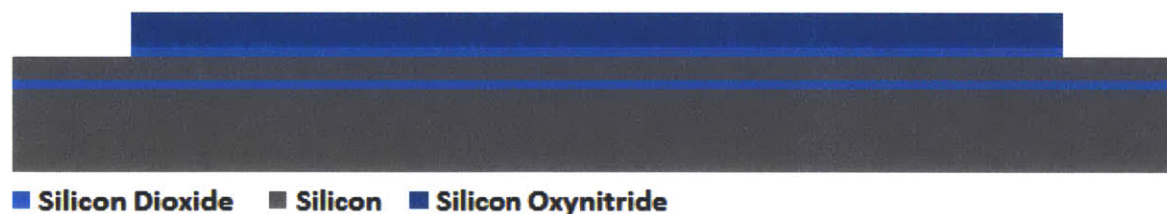
Figure 32 - The core and lower cladding are lithographically defined
