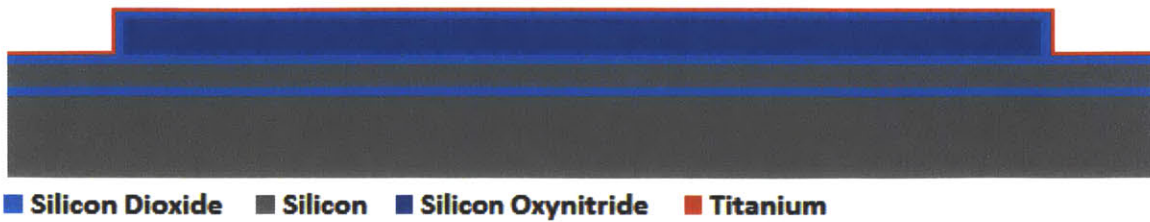
Figure 36 - A layer of titanium is sputtered to provide highly-reflective surfaces off which light can reflect in the case of corner-mirrors.
