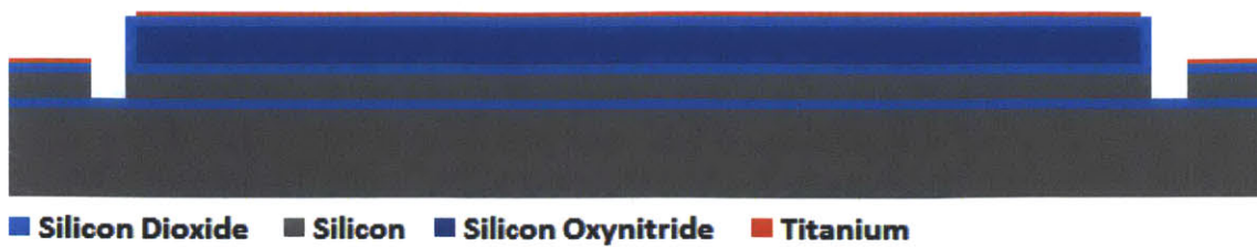
Figure 48 – The device layer is etched through to the buried oxide layer.
