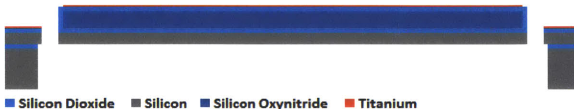
Figure 5 - The buried oxide layer is etched in a hydro-fluoric acid vapor. The wafer is subsequently released in a solvent bath.
