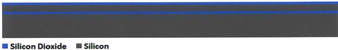
Figure 30 - Lower cladding deposited
