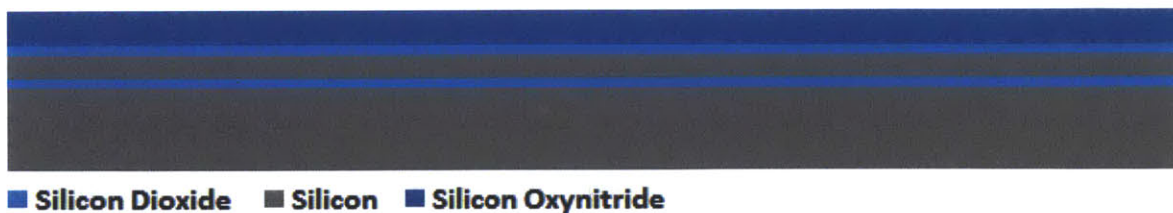
Figure 31 - Core (silicon oxynitride) deposited
