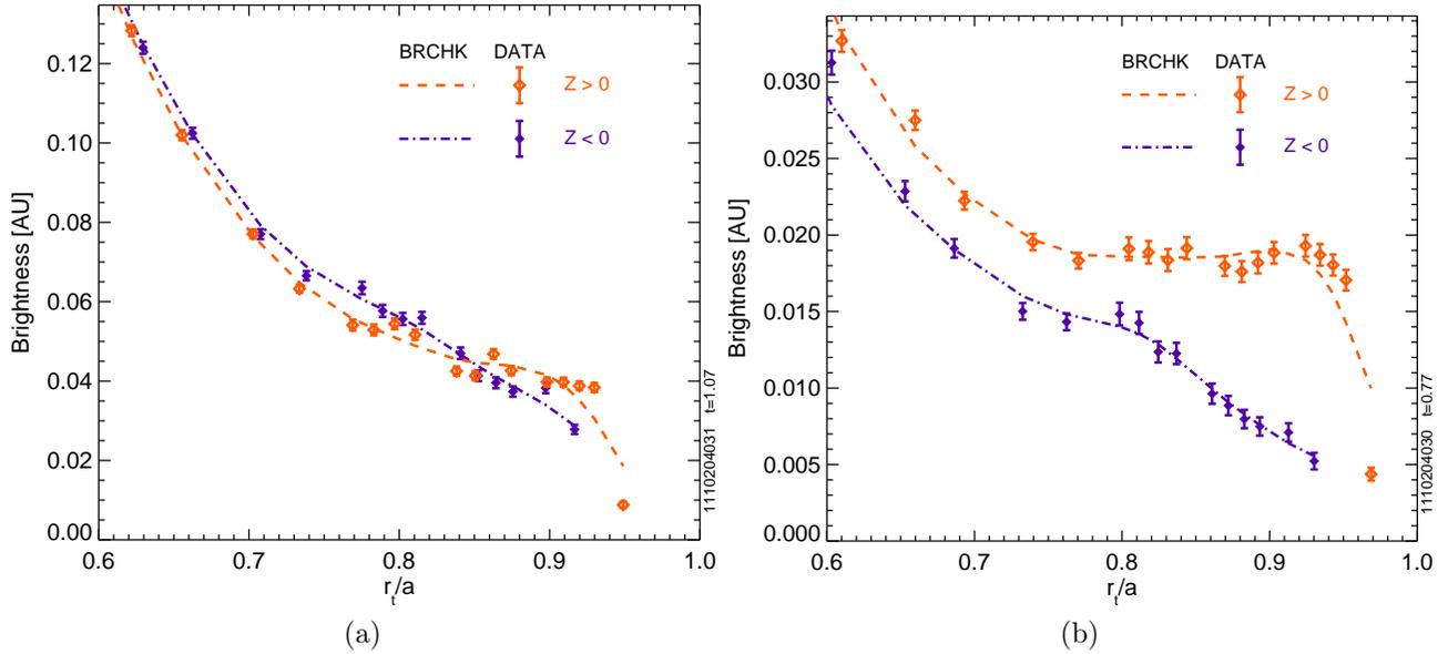
Figure 6: Brightness profiles showing weak or negligible up/down asymmetry in a 1.0 MA, 5.4 T plasma at  $\bar{n}_e \simeq 0.6 \times 10^{20} \text{ m}^{-3}$  (a) and a strong up/down asymmetry in a 0.6 MA, 5.4 T plasma at  $\bar{n}_e \simeq 0.5 \times 10^{20} \text{ m}^{-3}$  (b)
