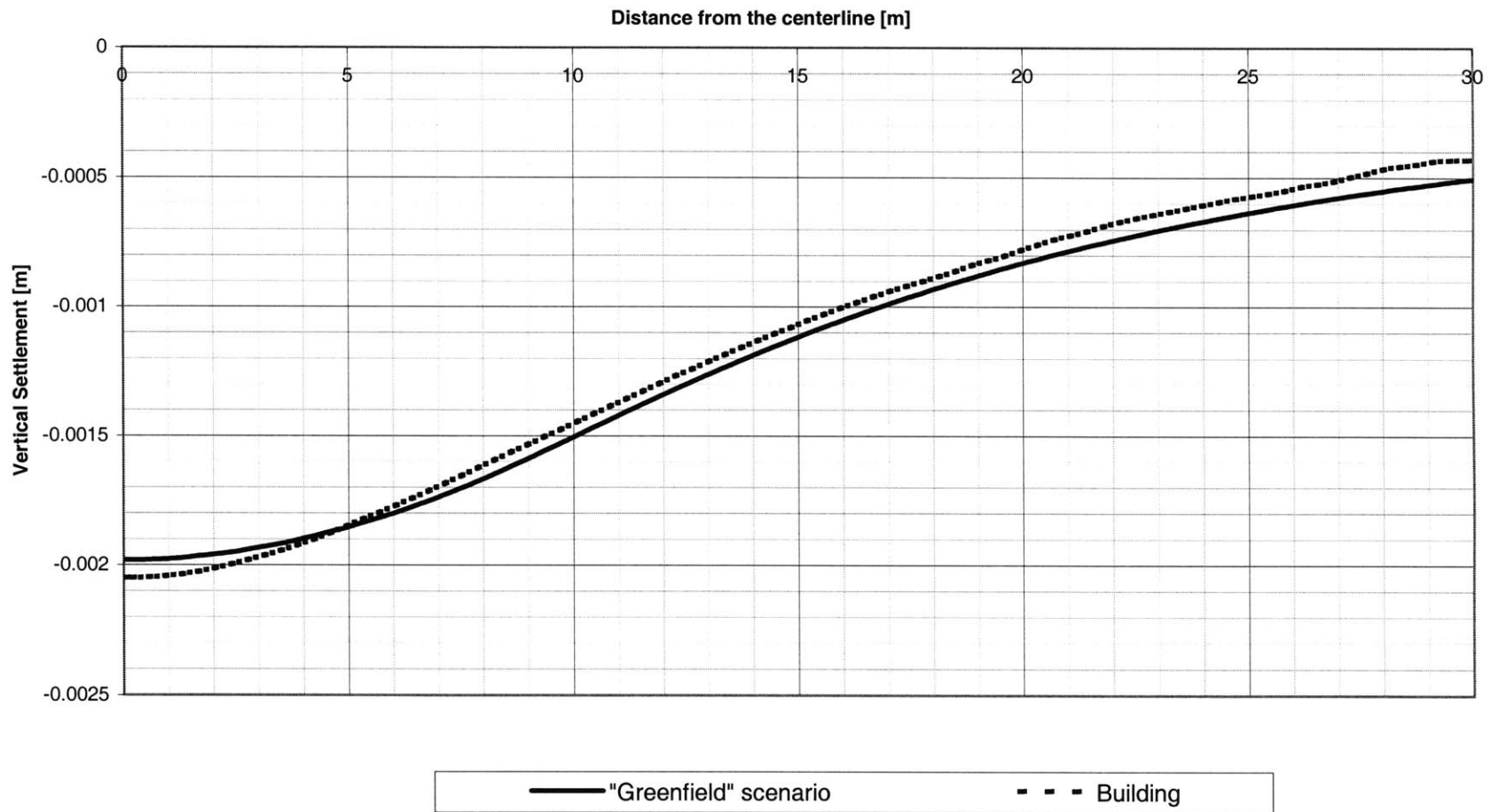
Figure 4.13. Comparison of settlement troughs for "greenfield" condition and a scenario with a structure that exhibits large \alpha^* and low \rho^* in undrained conditions
