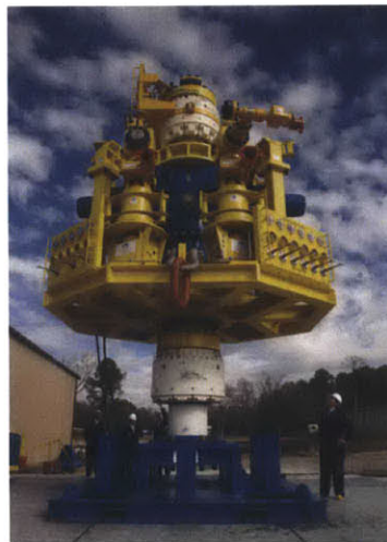
Figure A-2: Capping stack developed by Marine Well Containment Company
