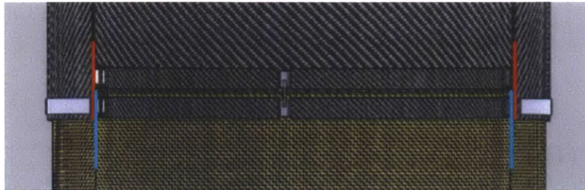
Figure 4-2: Connection of two consecutive shroud sections using shackles that are attached to the flanges connecting the 120 degree circular I-beam ribs.
