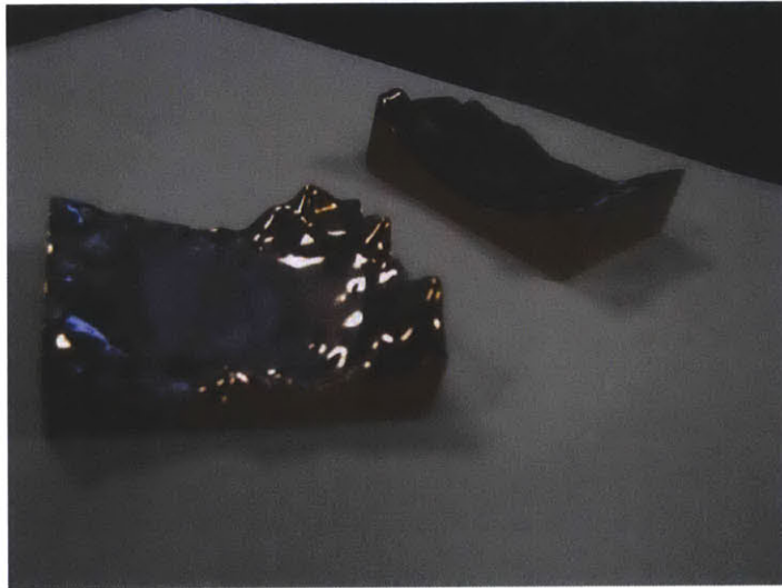
Figure 5-7: Photograph of copper mirror 1 (background) and mirror 2 (foreground). Mirrors were machined by Ramco Machine, LLC and the picture shows the interesting profiling of the phase correcting surface.
