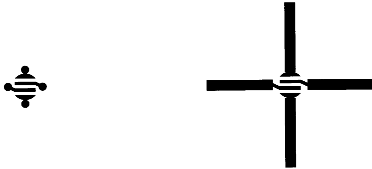
Figure D.2: First iteration of HHV5.0 ETS electrode patterns. Left - Piezo electrodes; Right - Silver electrodes. The piezo electrodes made contact with the brass rods through four 0.03 inch diameter circular extensions Figure D.2, and the total active area of each piezo electrode was 0.63 \text{ mm}^2 . The subsequent design took advantage of the empty areas not utilized by making the contact a subportion of the electrode, increasing the area per electrode. Compare to Figure 5.3.
