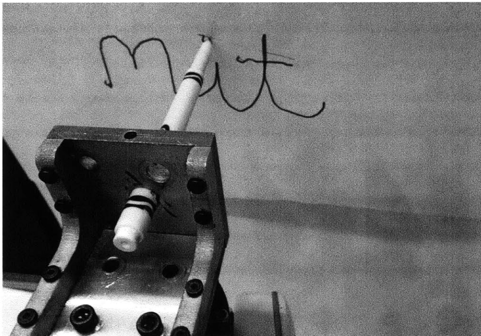
Figure 13. Close up of writing done with marker using real time control for the robotic arm via the gui sketchpad.
