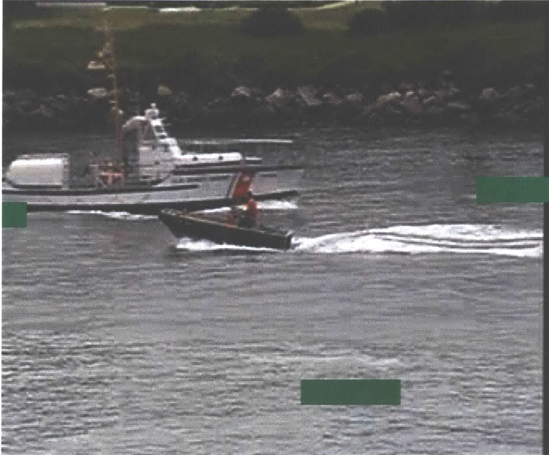
Figure 3-1: I-frame #48 from the “coastguard” stream with packet loss. Y PSNR = 21.995697
