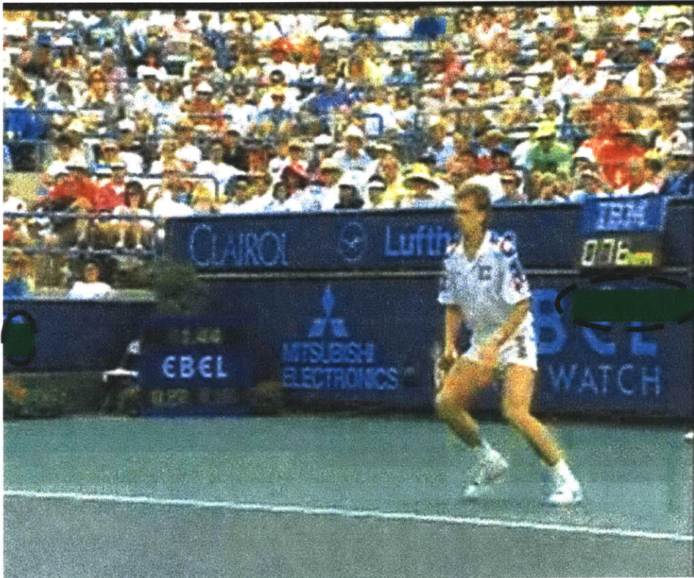
Figure 3-16: I-frame with Packet Loss. Packet loss is visible in the area above the “watch” advertisement. This error will propagate to subsequent frames if not corrected.
