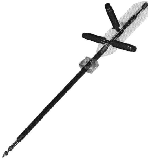
Figure C-2: A more fully fleshed out version, including motors at the base, a universal joint near the tip, and a 3-axis force sensor behind the blunt probe. Position sensing in this version is done with the encoders on the motors, but redundant sensors closer to the tip would improve accuracy.
