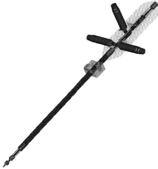
Figure 7-2: Concept for large-scale, 3-D motion force-displacement probe, the TeMPeST 3-D.
