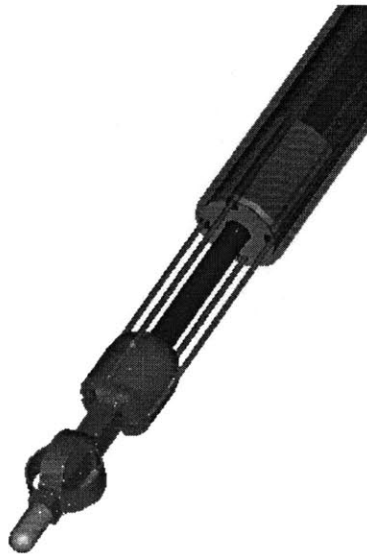
Figure C-3: Tip design for the TeMPeST 3-D. A universal joint permits motion in pitch and yaw, but prevents rotation of the tip about the shaft. Linear bearings in the sleeve support the axial motion of the tip. A novel 3-axis force sensor (pitch- and yaw-moment, and axial thrust) measures the reaction forces of the tissue.
