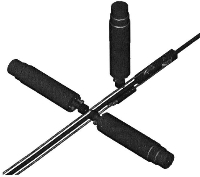
Figure C-4: Cable drive system for the TeMPeST 3-D. The top motor controls pitch of the probe, the side motors are redundant in controlling yaw, and all together they move the central carriage along the shaft of the tool. Not shown are linear bearings which would support the shaft at the upper right, and lower left, as well as at the tip of the tube (see figure C-2).
