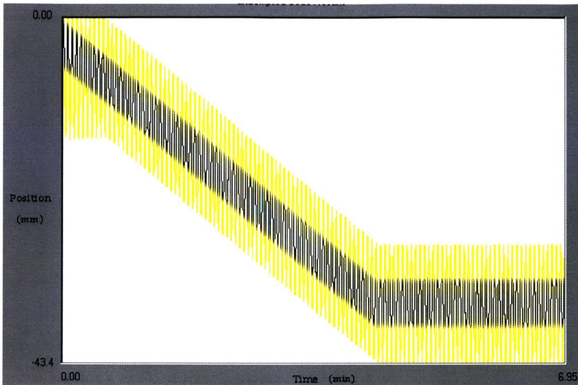
Figure B-5. Tracking data of moving LED to demonstrate tracking algorithm effectiveness.
