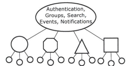
Figure 4.13: The intermediate iteration of the InterTwinkles architecture: central group server handling authentication, groups, search, events, and notifications; but distinct servers handling different communications tools (e.g. Dotstorm, Points of Unity, etc.)
