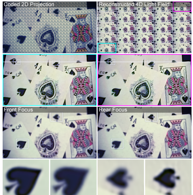
Figure 10: Light field reconstruction from a single coded 2D projection. The scene is composed of diffuse objects at different depths; processing the 4D light field allows for post-capture refocus.
