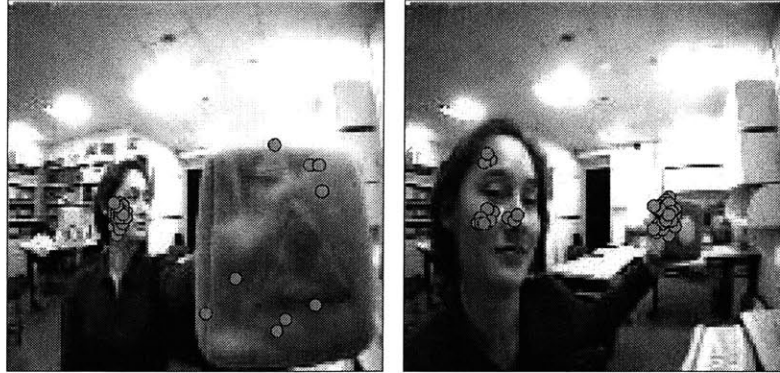
Figure 6-3: Effect of gain adjustment on looking preference. Circles correspond to fixation points, sampled at one second intervals. On the left, the gain of the skin tone filter is higher. The robot spends more time looking at the face in the scene (86% face, 14% block). This bias occurs despite the fact that the face is dwarfed by the block in the visual scene. On the right, the gain of the color saliency filter is higher. The robot now spends more time looking at the brightly colored block (28% face, 72% block).
