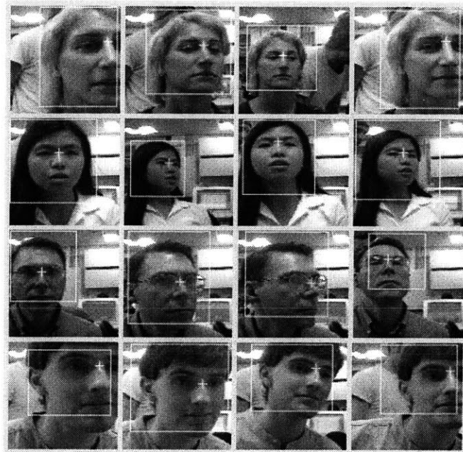
Figure 6-5: Sequence of foveal images with eye detection. The eye detector actually looks for the region between the eyes. It has decent performance over a limited range of distances and face orientations. The box indicates a possible face has been detected (being both skin toned and oval in shape). The small cross locates the region between the eyes.
