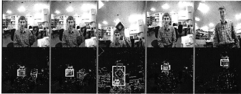
Figure 6-9: Manipulating the robot's attention. Images on the top row are from Kismet's upper wide camera. Images on the bottom summarize the contemporaneous state of the robot's attention system. Brightness in the lower image corresponds to salience; rectangles correspond to regions of interest. The thickest rectangles correspond to the robot's locus of attention. The robot's motivation here is such that stimuli associated with faces and stimuli associated with toys are equally weighted. In the first pair of images, the robot is attending to a face and engaging in mutual regard. By shaking the colored block, its salience increases enough to cause a switch in the robot's attention. The third pair shows that the head tracks the toy as it moves, giving feedback to the human as to the robot's locus of attention. The eyes are also continually tracking the target more tightly than the neck does. In the fourth pair, the robot's attention switches back to the human's face, which is tracked as it moves.
