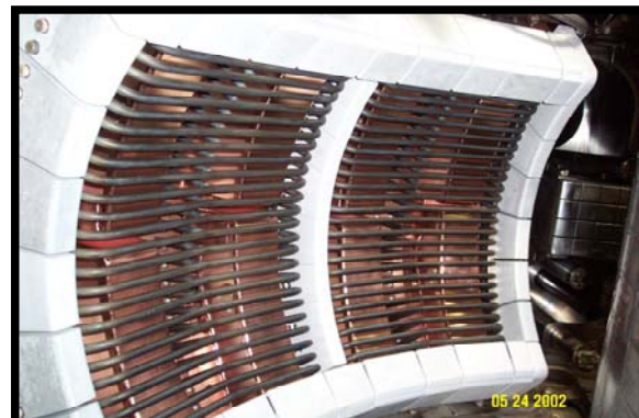
FIG. 2. Four strap fast wave antenna installed at J-port.
