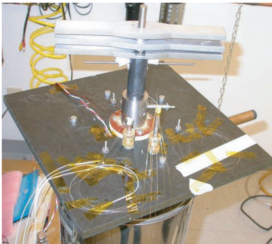
Figure F-7: Top view of the probe showing the threaded rod with the pulling mechanism.
