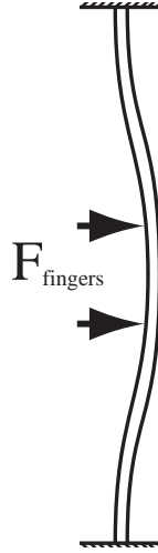
Figure E-3: The bending of a cylinder section that is held fixed at both ends.
