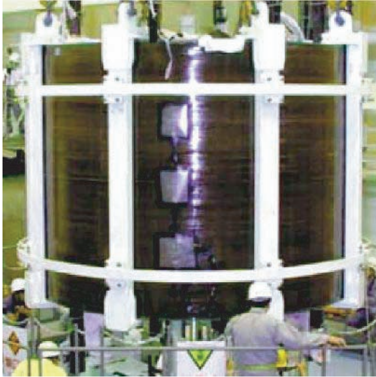
Figure 1-11: The ITER CS model coil achieved a maximum field of 13.5 T, with a maximum current of 46 kA, and a stored energy of 640 MJ.
