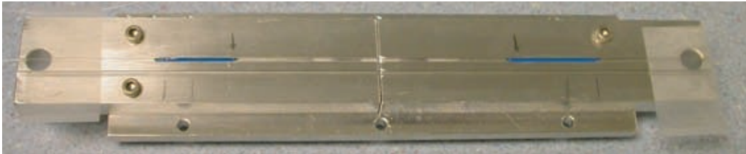
Figure A-1: Fiber holder that slides apart to strain the fibers. The section of the fiber between the blue Stycast epoxy will be strained.
