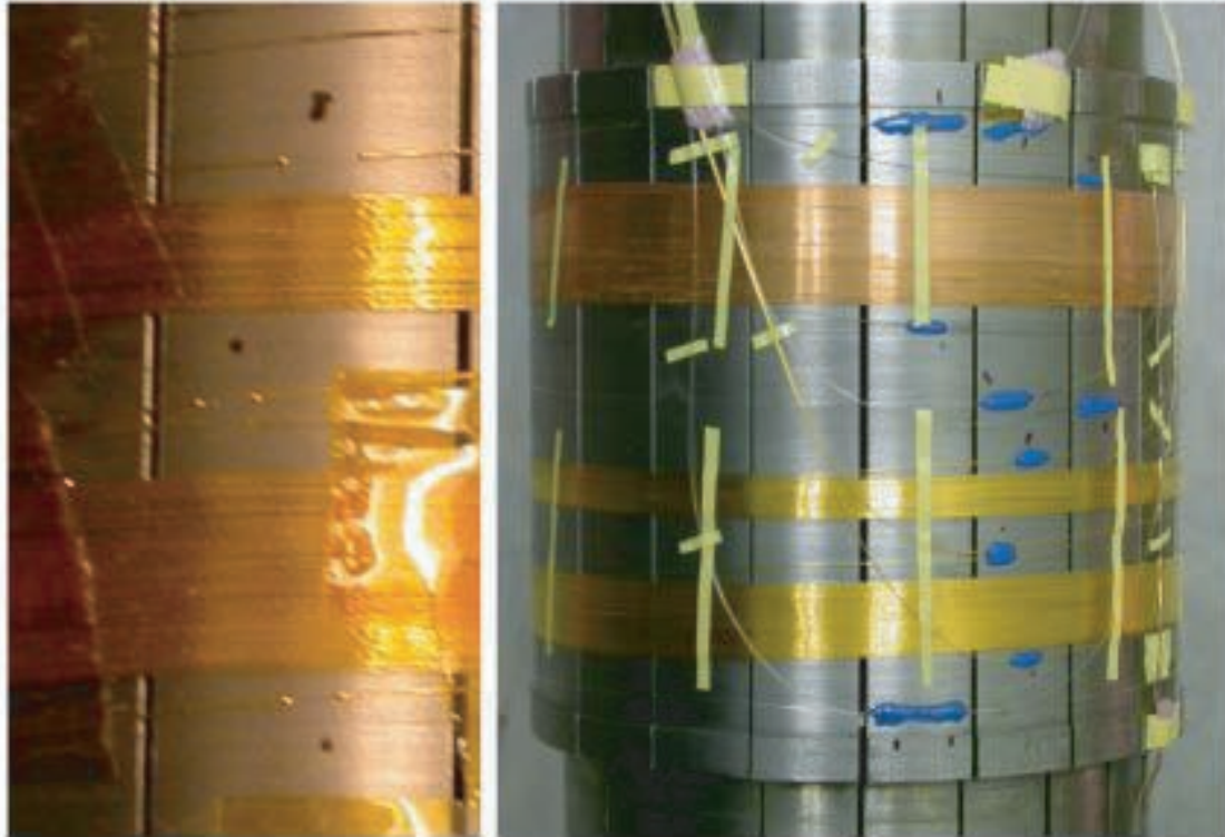
Figure F-6: Gold coating stripped off fibers where they will be epoxied (left), and the sample fiber epoxied into place (right).
