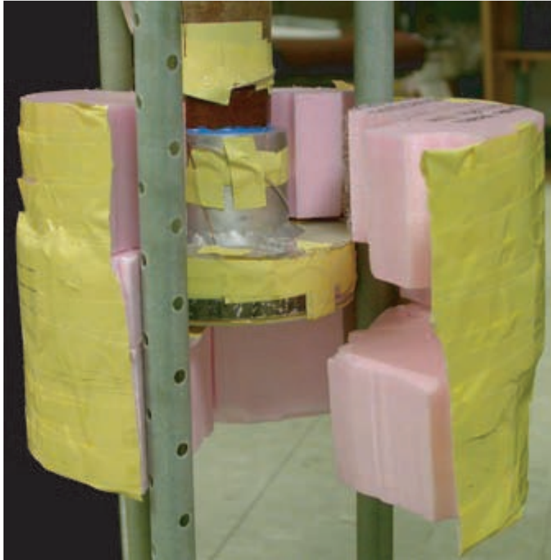
Figure C-3: Sample fiber holder with its Styrofoam insulation.
