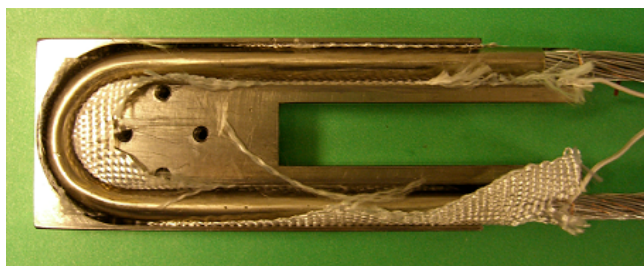
Fig. 4.6 U-shape holder. Only the 45-strand cable required a supporting titanium tube in the bending area. sample in its
