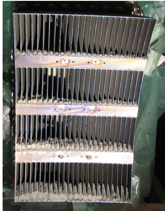
Figure V-2: In the 2005 Alcator C-mod tokamak campaign, the lower hybrid launcher experienced corrosion by hydrogen and deuterium, spewing titanium dust across the machine. (a) Dust particles in visible light (red dots), as they radiate before eventually melting. (b) Dust deposited on the launcher after plasma operation.
