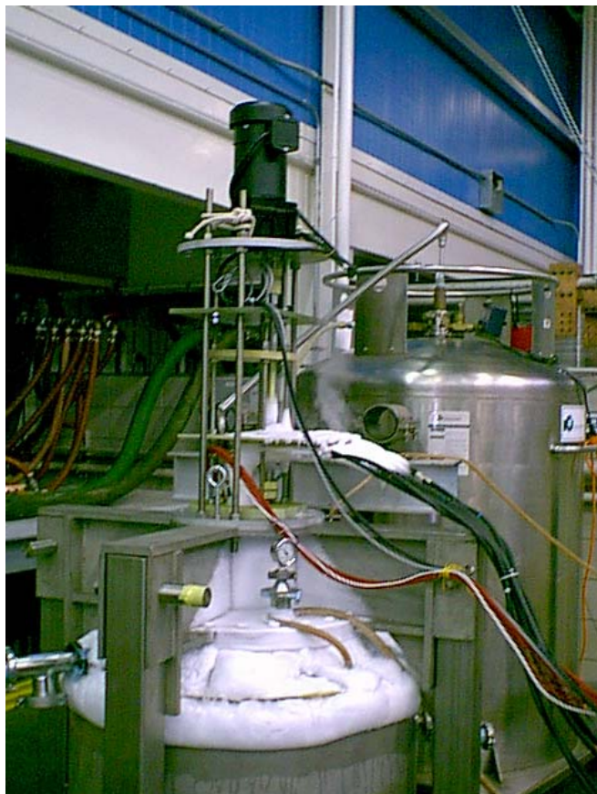
Fig. 6 The test probe with a gear driver motor is mounted from the top of the cryostat
