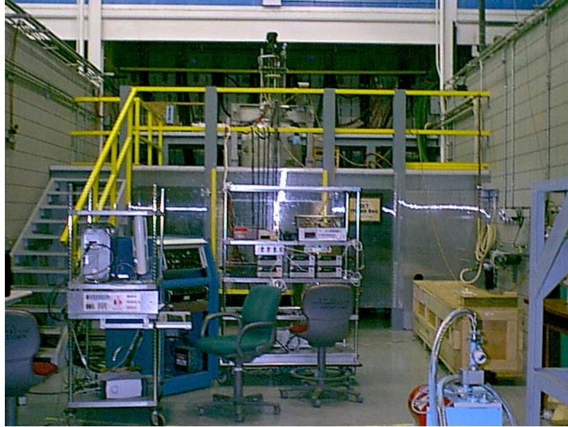
Fig. 5 Pure bending test set up in the 20 T, 195 mm Bitter magnet cell at NHMFL.
