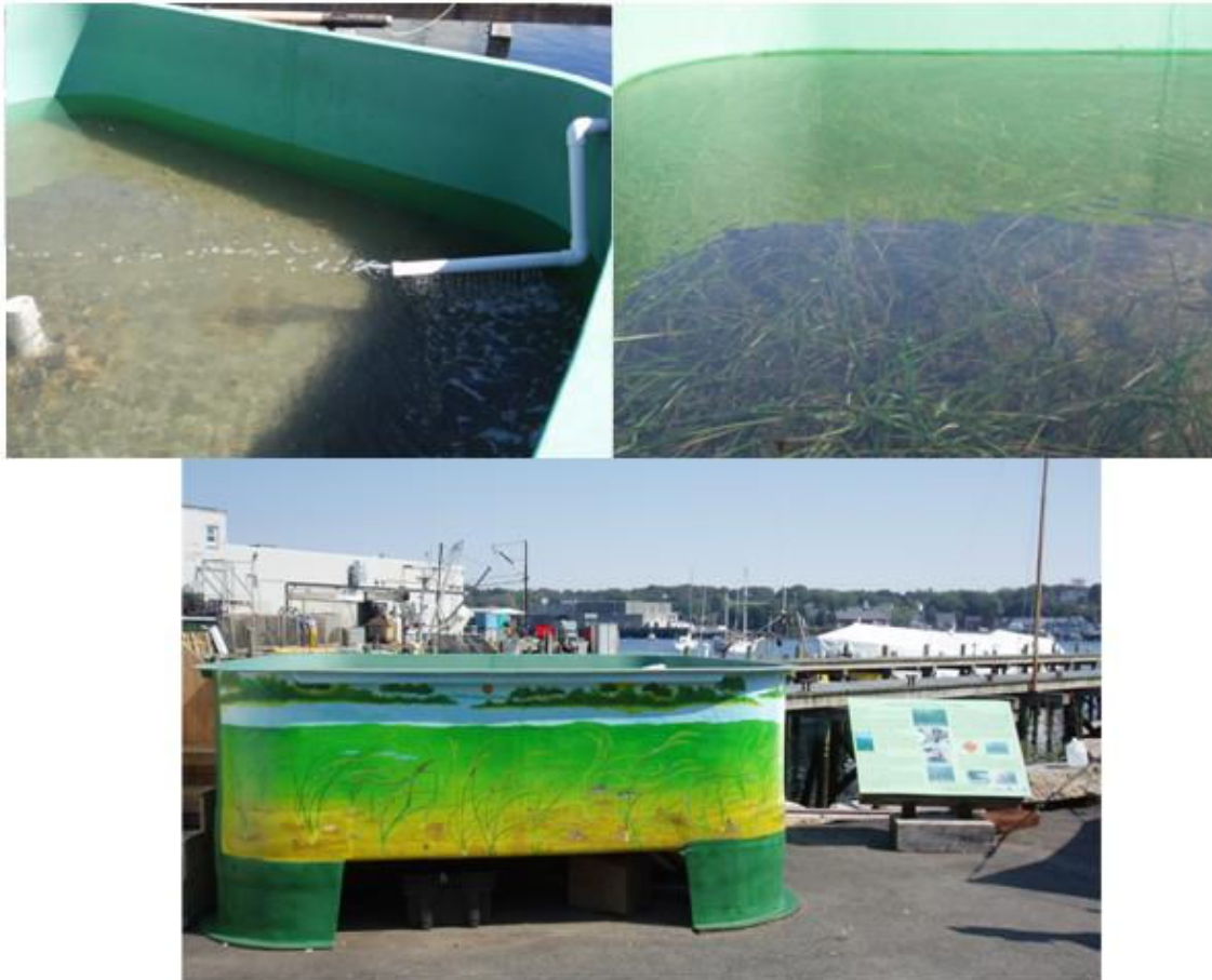
FIGURE 6. Flow-through tank at GMHC, showing (clockwise from top left) water flow with center standpipe, planted eelgrass, and tank with mural of eelgrass habitat and adjacent informational poster.
