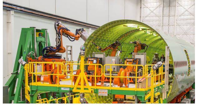
Fig. 1: The Boeing Fully Autonomous Upright Build for the Boeing 777. Image courtesy of Boeing Research and Technology.
