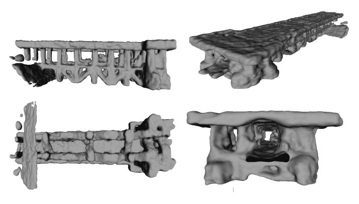
Figure 15: The mesh-based high quality map for the above-water part of the jetty, using a low probability threshold for occupied cells and the Poisson surface reconstruction algorithm. Cell-size=8cm.
