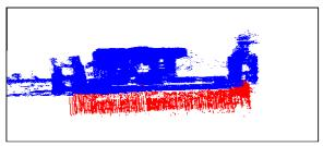
(b) Above- and below-water parts of marine structure, point cloud-based map. In red color below water part, in blue color above water part.
