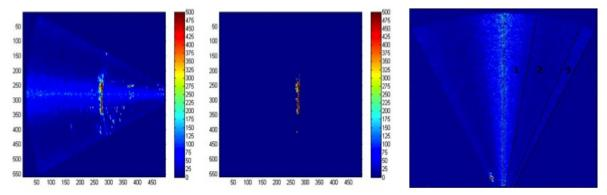
(a) In the left figure we can see a frame of raw noisy sonar data, in the figure in (b) An empty sonar frame divided into the right we can see the filtered sonar data using a filter based on clustering. 6 clusters.
