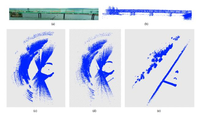
Figure 10: Reconstruction of a jetty in Pandan Reservoir, Singapore. (a) The target jetty. (b) Side view of the jetty model constructed by our algorithm. (c) Top view of multiple frames of the 3-D LiDAR data before processing. (d) Top view of the constructed 3-D model based on GPS and compass information. (e) Top view of the constructed 3-D model generated by our algorithm.
