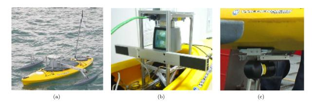
Figure 2: (a) The ASV with Velodyne LiDAR mounted on top of it. An additional pontoon is attached to the ASV to improve stability of the ASV. (b) The Velodyne LiDAR and the mounting platform for placing the LiDAR in an inverted configuration on the ASV. (c) The BlueView MB2250 micro-bathymetry sonar mounted in a sideways configuration.
