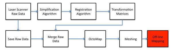
Figure 4: The off-line map: Less simplified data are used to get vehicle's trajectory and then vehicles' trajectory is used to project raw data resulting a dense point cloud.
