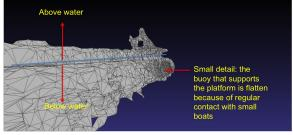
(c) Above- and below-water parts of marine structure, point (d) Above- and below-water mesh-based map: Small details. cloud-based map. In red color below water part, in blue color above water part.
