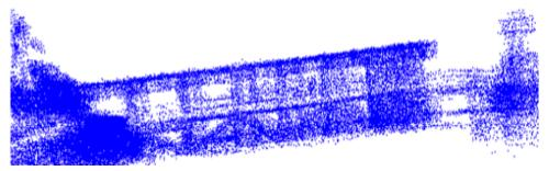
(b) Low-resolution map, cell size= 30cm, the mission lasts 3mins, is generated in 3mins (3GHz CPU).
